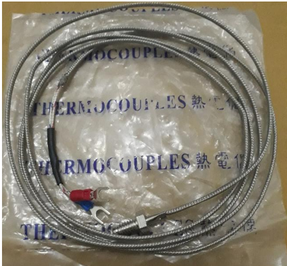
Gambar 3.6 Thermocouple type K
