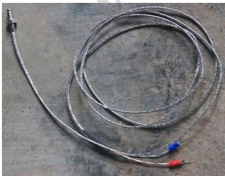
Gambar 3.9 Thermocouple
