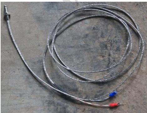
Gambar 3.9 Thermocouple
