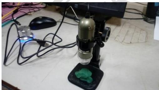
Gambar 3.16 Dino Lite Digital Microscope
