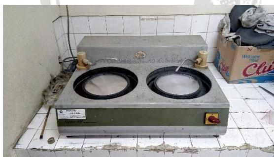
Gambar 3.14 Centrifugal Sand Paper Machine
