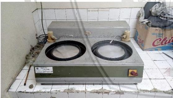
*Gambar 3.14* Centrifugal Sand Paper Machine
