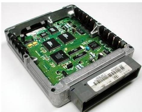
Gambar 2.9 *Engine control unit*
