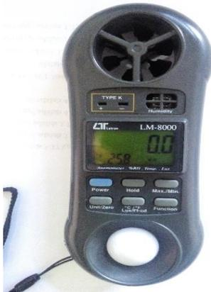
Gambar 3.2 Anemometer digital
