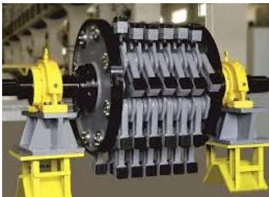
Gambar 2.8 *Heavy Duty Hammer Shredder (HDHS)*
