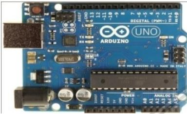
Gambar 2.15 Board Arduino Uno berbasis ATmega 328P
