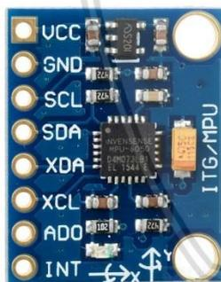
**Gambar 2.12** MPU6050 *Module*
