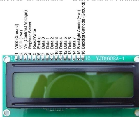
Gambar 2.14 Pinout modul LCD teks
