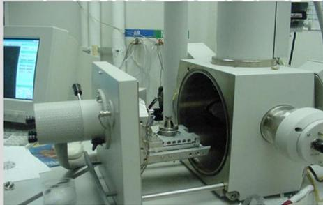
**Gambar 2.3** Instrumen *Scanning Electron Microscopy* (SEM)
