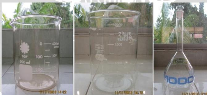
**Gambar L.11** Beaker glass 500 ml, 2000 ml, dan labu erlemeyer 1000 ml
