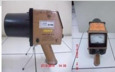
**Gambar 2.5** Surveimeter Beta Gamma
