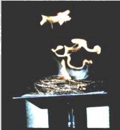
**Gambar 2. 4** Fase flaming combustion
