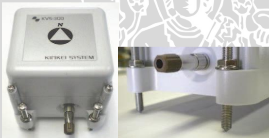
Gambar 3.2 Seismometer KVS-300 (Triastuty, 2010)
