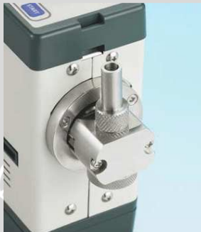
Gambar 3.6: Impactor piezobalance dust monitor kanomax model 3522
