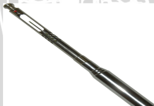
Gambar 3.10: Straight probe kanomax anemomaster model A031
