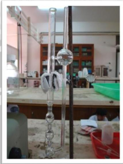
**Gambar I.5 Alat Viskometer Canon-Fenske 350**
