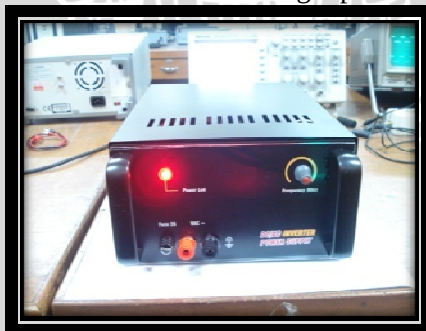
DC/AC power inverter
