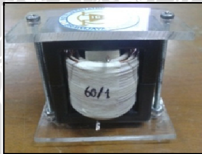
Gambar 4.3 Transformator matching impedance (Susanto, 2012)
