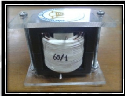
Transformator matching impedance
