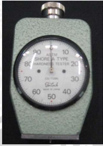
Gambar 3.5. Shore A Durometer
