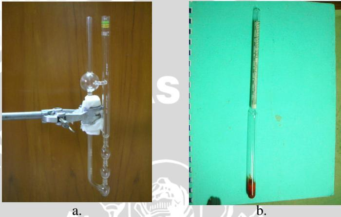
**Gambar 3.3** (a) Viskometer oswald (b) Arhoemeter
