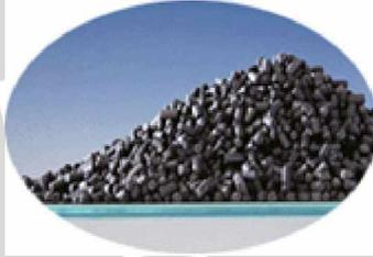
**Gambar 2.5** Pelleted activated carbon.
