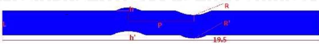
Gambar 3.1 Geometri *Corrugated Metal Gasket 25A*
