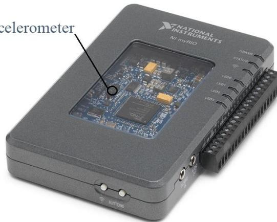
**Gambar 2.2** Sensor on board accelerometer myrio
