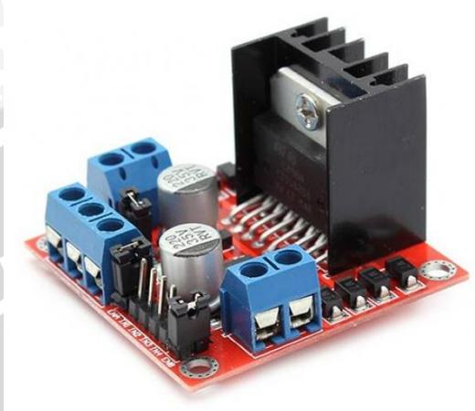
**Gambar 2.8** Driver motor L298N dual H-Bridge
