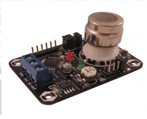
**Gambar 2.9 MG-811 CO<sub>2</sub> Gas Sensor**
