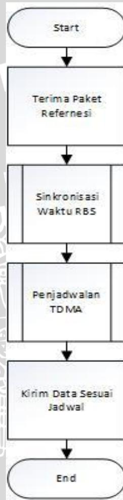
**Gambar 5.9** Diagram Alir Node Receiver
