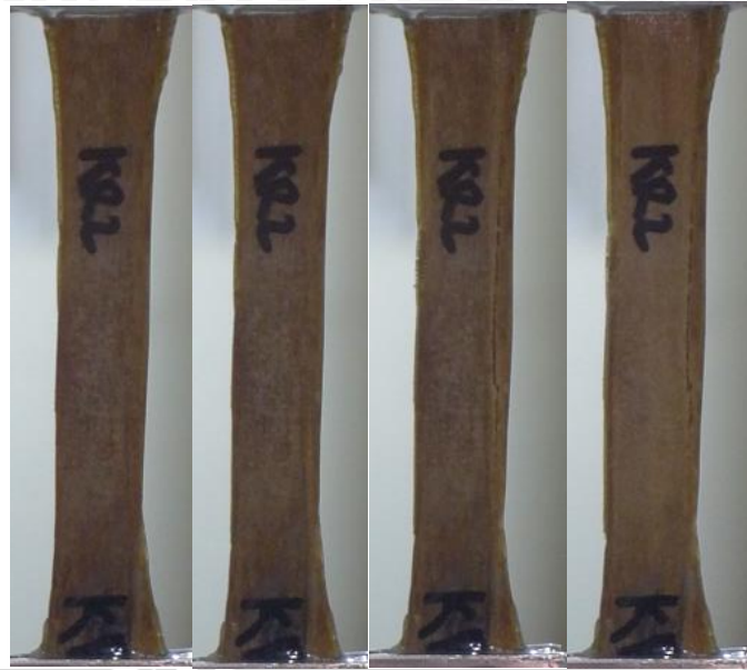
Gambar 4.16 Fase patahan specimen Uji Tarik matrik Ripoxy
