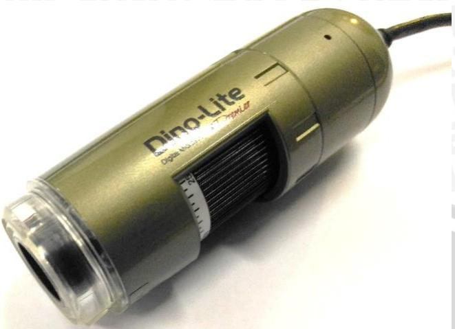
Gambar 3.5 Kamera Dino-lite microscope
