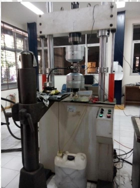
Gambar 3.3 *Hydraulic servo pulser*
