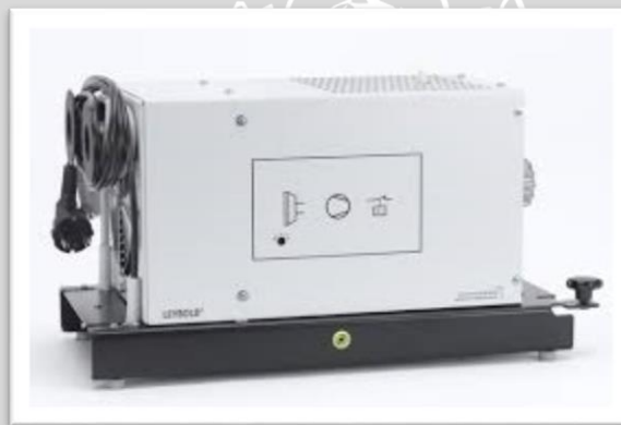
Gambar 2.2 Magnetic Powder Brake 1 kW (Sumber: Leybold)
