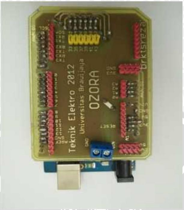
Gambar 1.1 *Shield Board* Arduino Mega 2560
