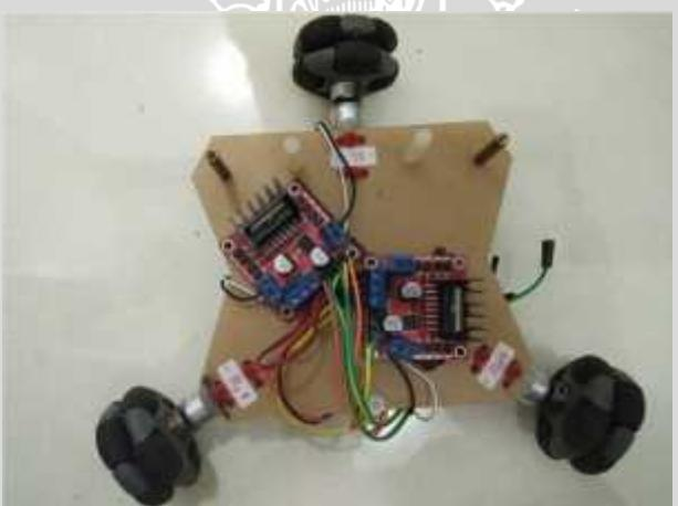
Gambar 1.2 Body Bawah, Modul Driver L298N, Motor DC, dan *Omni Wheel*
