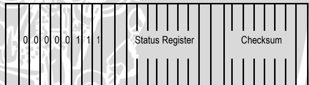
Figure 15: Status Register Read
