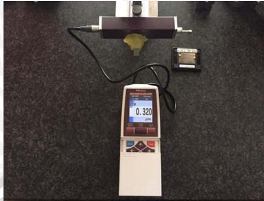
Gambar 3.5 *Surface roughness tester* Mitutoyo SJ-210
