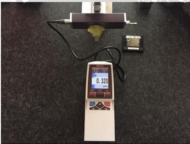
Gambar 3.4 *Surface roughness tester*.
