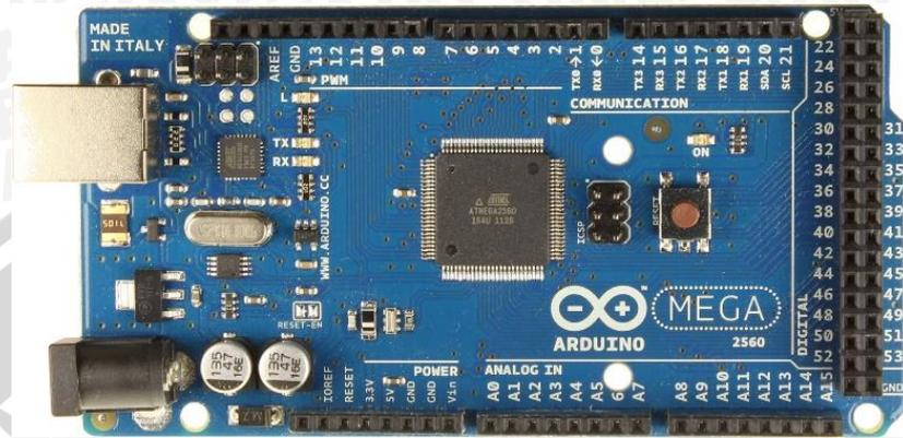
Gambar 6.3 Board Arduino Mega 2560.
