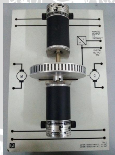
Gambar 3.15 Plant motor generator DC 73411
