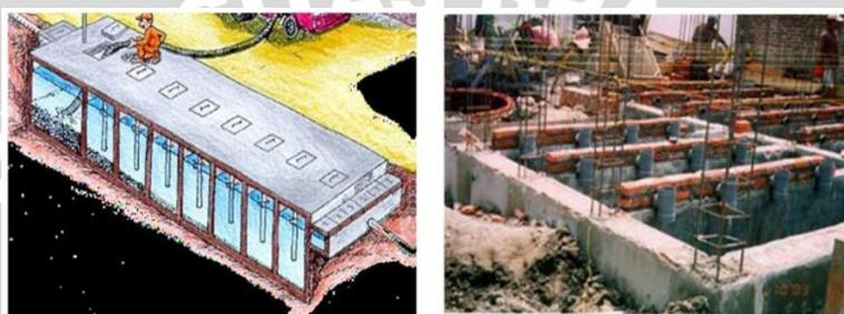
Gambar 2. 2 *Baffled Reactor*
