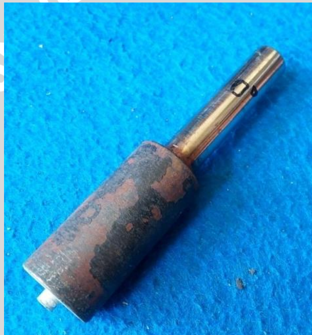
Gambar 3.7 Tool Pengelasan 0^\circ S45C
