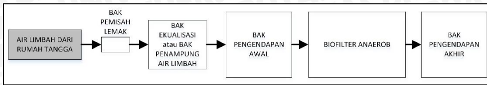
Gambar 4.25 Diagram Proses Pengolahan Air Limbah Aerob dan Anaerob Sumber: Said, 2008
