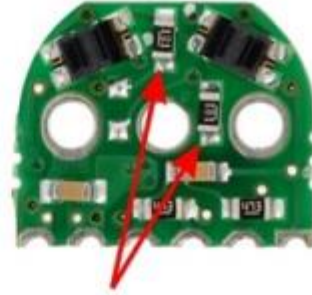
two current-limiting resistors (IR LEDs in parallel)
