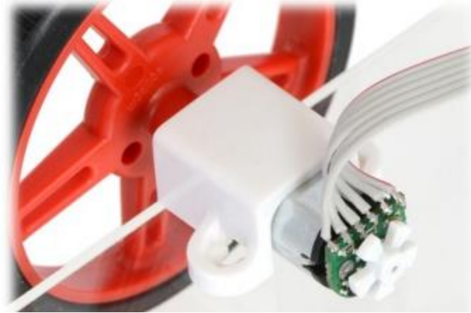
Example of an installed micro metal gearmotor reflective optical encoder.
