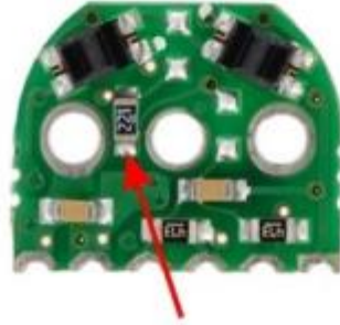
one current-limiting resistor (IR LEDs in series)
