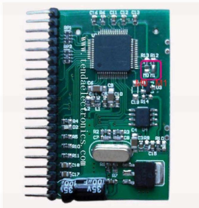
**MP3 Mode :** The module will work as a normal mp3 player with Play/Pause , Stop,Prev.,Next, FF 10 (Fast forward 10 songs),REW 10 (Rewind 10 songs), Vol+,Vol- functions .
