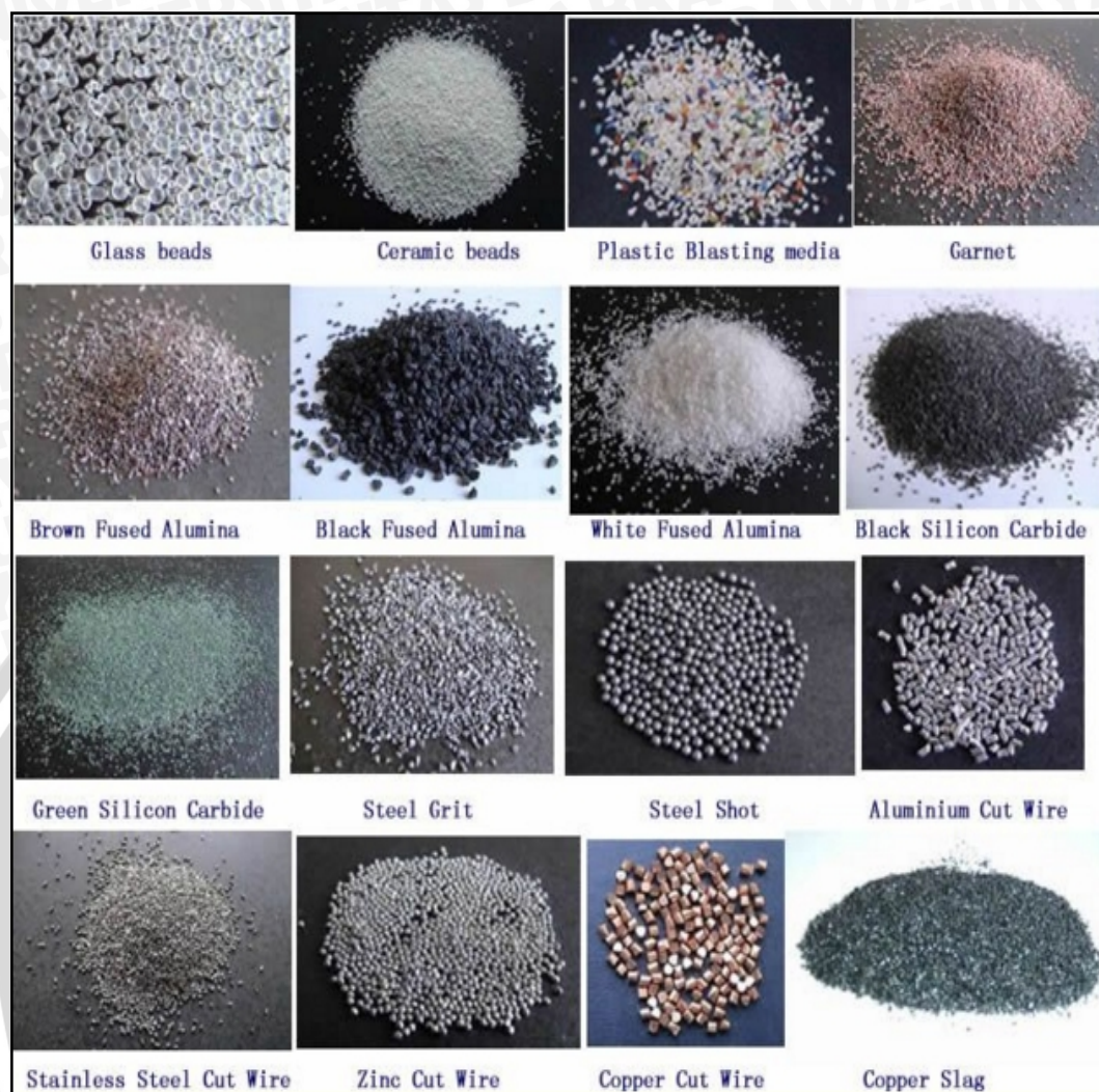
Gambar 2.6 Macam macam material abrasif sandblasting
