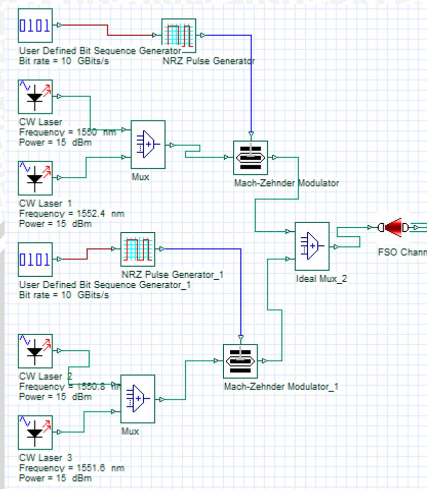
**Figure 4.19** Non Chirped NRZ Transmitter Scheme
