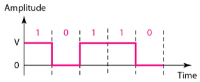
**Figure 2.5** Unipolar NRZ Signal
