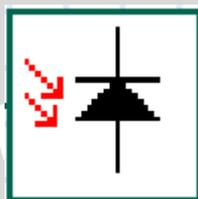
**Figure 4.12** Photodetector PIN
