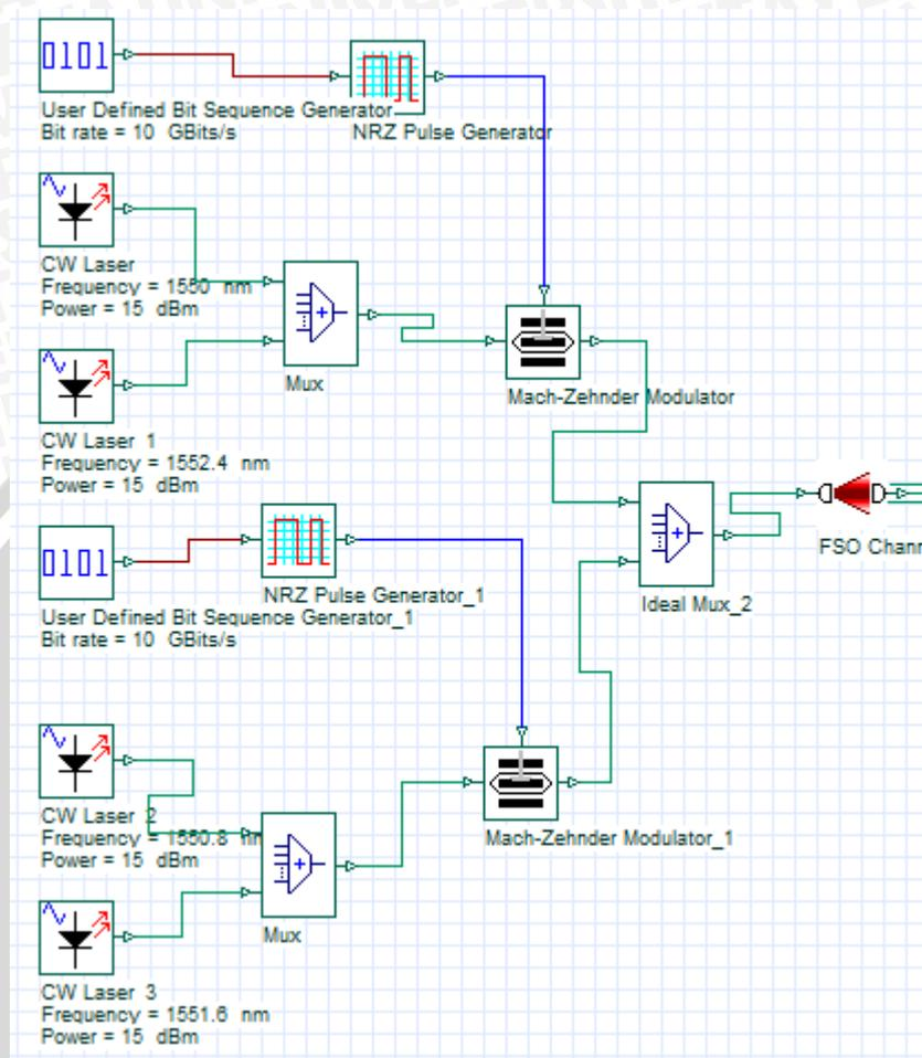
**Figure 4.19** Non Chirped NRZ Transmitter Scheme
