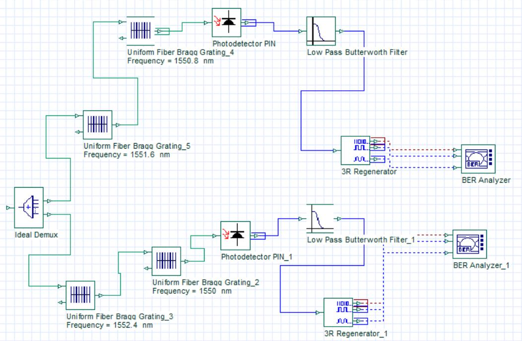
**Figure 4.22** Receiver Scheme for Non Chirped NRZ, Chirped NRZ, and RZ
