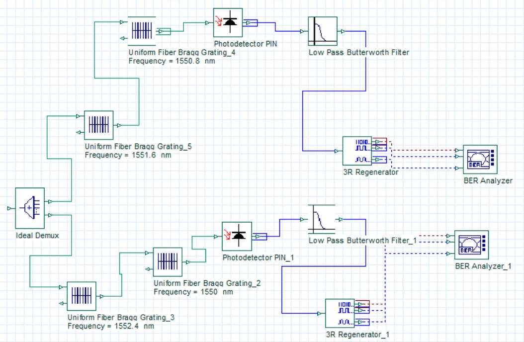
**Figure 4.22** Receiver Scheme for Non Chirped NRZ, Chirped NRZ, and RZ
