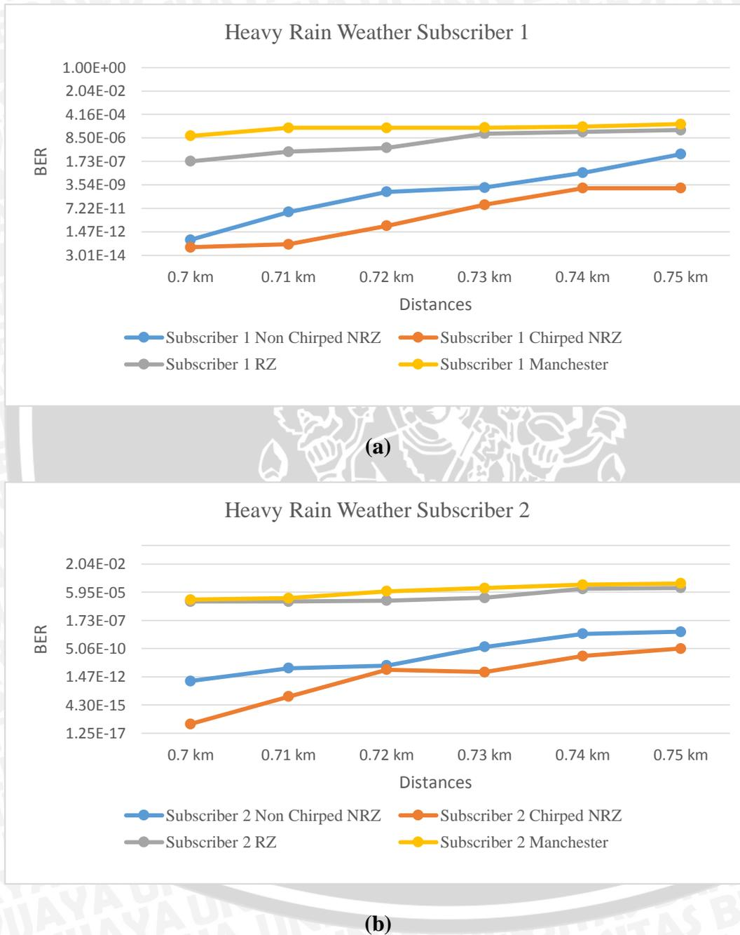
**Figure 4.30** (a) Distance Versus BER in Heavy Rain Weather for Subscriber 1 (b) Distance Versus BER in Heavy Rain Weather for Subscriber 2
