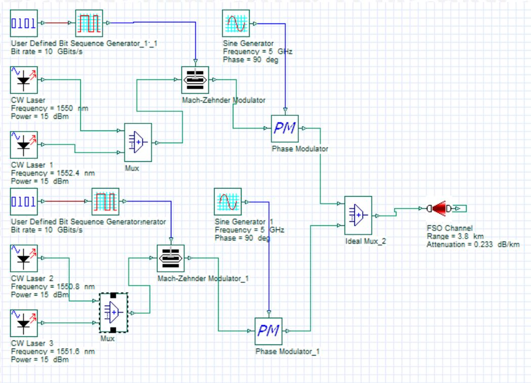
**Figure 4.20** Chirped NRZ Transmitter Scheme
