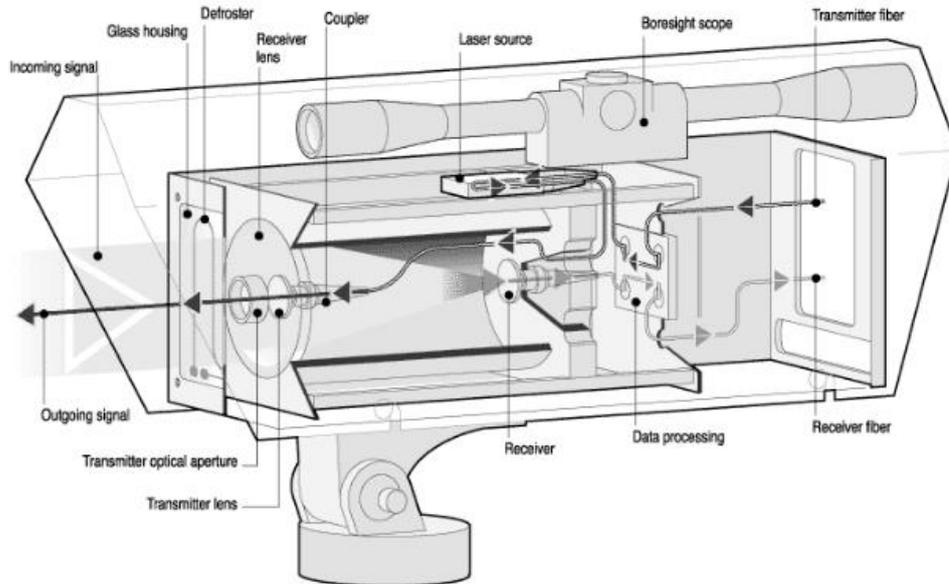
**Figure 2.2** Example Equipment for Free Space Optical Link
