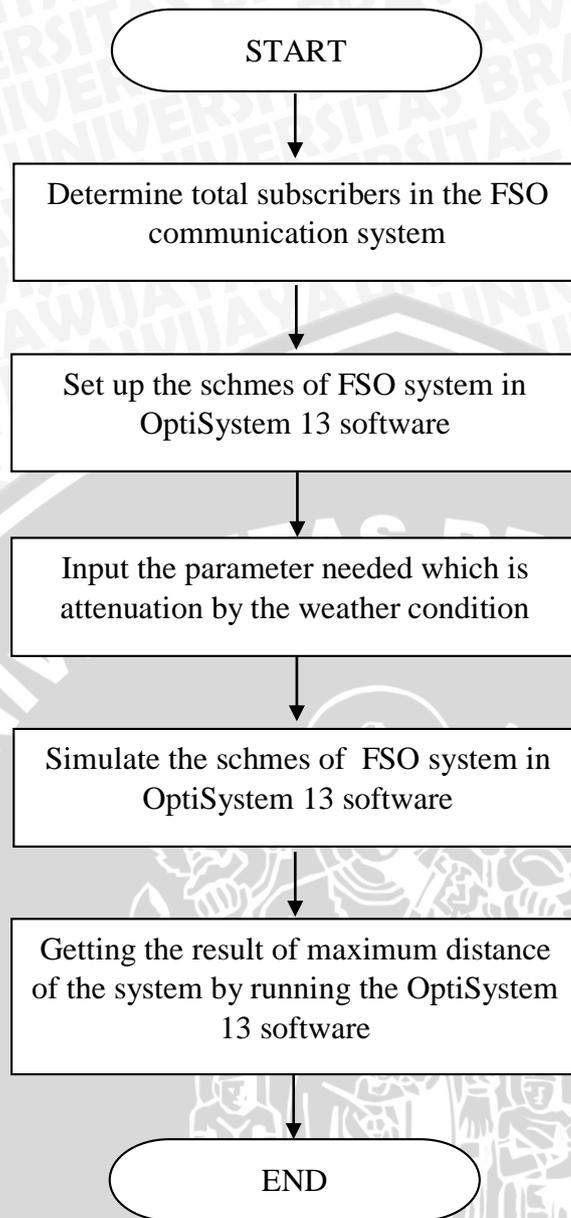
**Figure 3.1** Steps to Collect Primary Data
