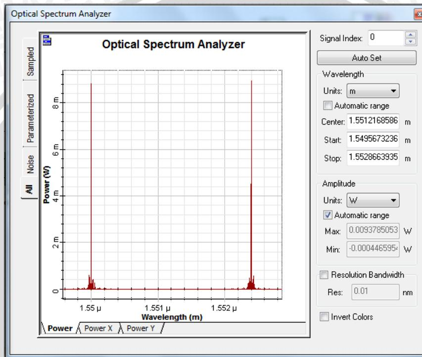
**Figure 4.31** Mach-Zehnder Modulator Output From NRZ system
