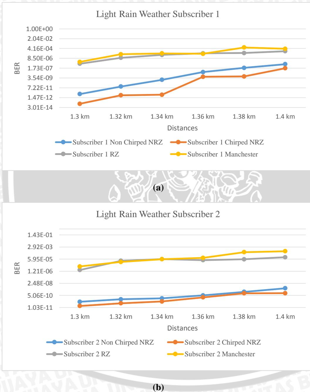
**Figure 4.28** (a) Distance Versus BER in Light Rain Weather for Subscriber 1 (b) Distance Versus BER in Light Rain Weather for Subscriber 2 (Source: Research)
