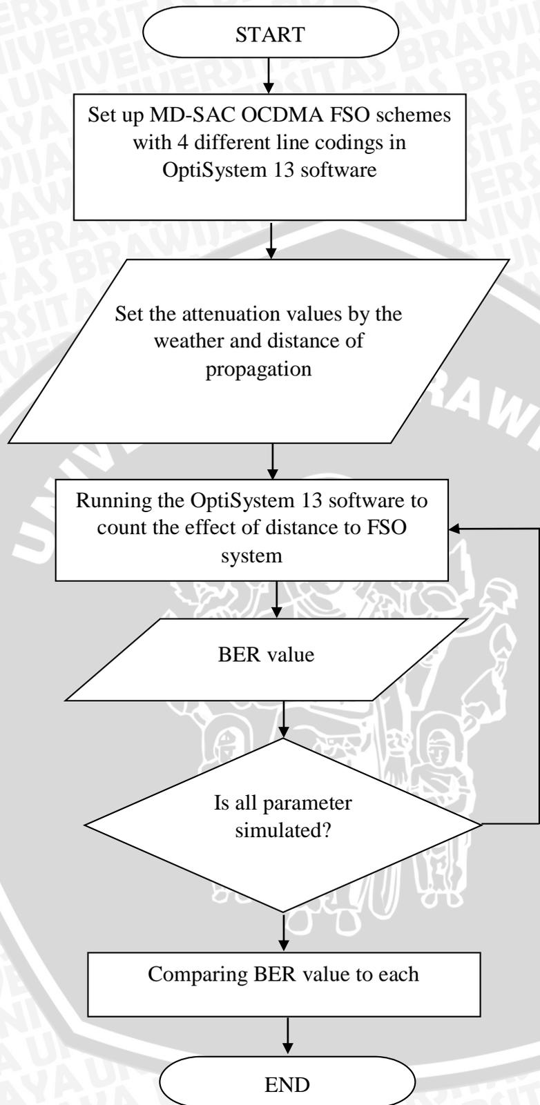
**Figure 3.3** Flow Chart of Distances effect to FSO System
