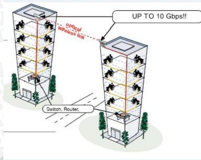
**Figure 1.1** Free Space Optical communication network between two buildings
