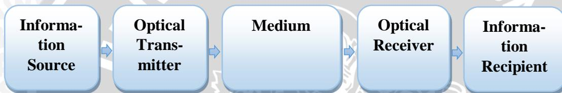
**Figure 2.1** Free Space Optical Communication Component
