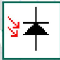
**Figure 4.12** Photodetector PIN
