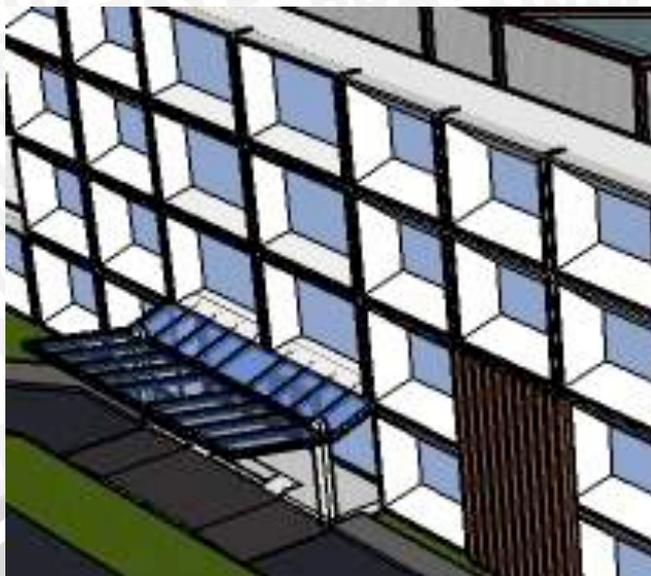
**Gambar 4.40** Penerapan *Shading Device*
