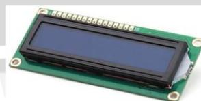
Gambar 2 Liquid Crystal Display
