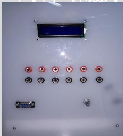
Gambar L 2. 2 Control unit magnetic powder brake tampak depan
