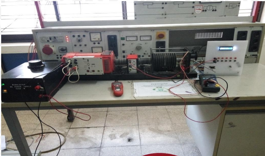
Gambar L. 2. 5 Rangkaian pengujian control unit magnetic powder brake
