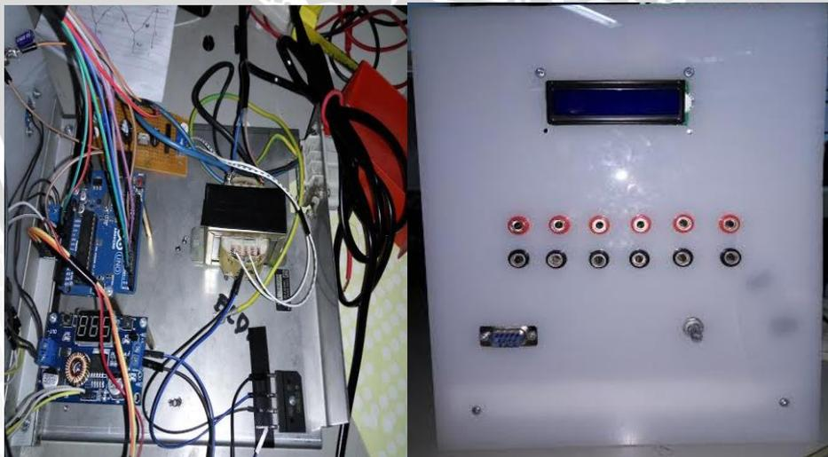
Gambar 4.2 *Control Unit Magnetic Powder Brake*
