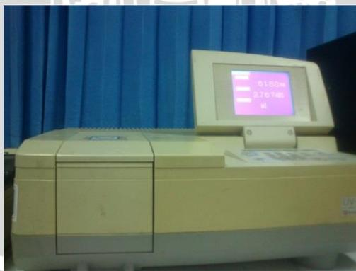
Gambar 5. 1 :UV-VIS Spectrophotometer (Shimadzu) tipe UV – 1601.
