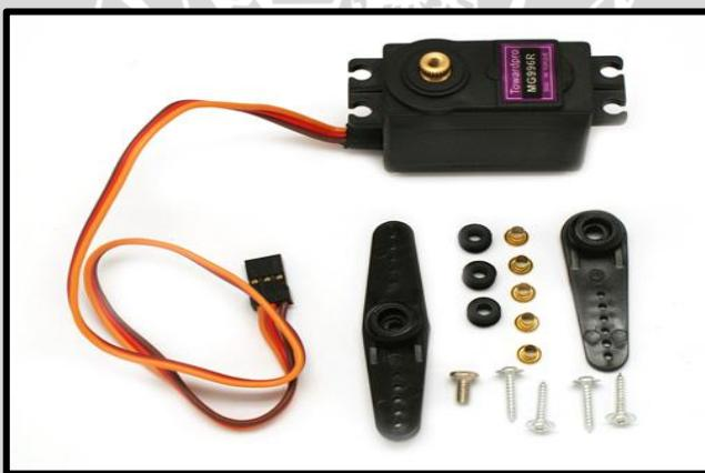
Gambar 4.8 Motor Servo Toward Pro MG996R (Perancangan, 2016)
