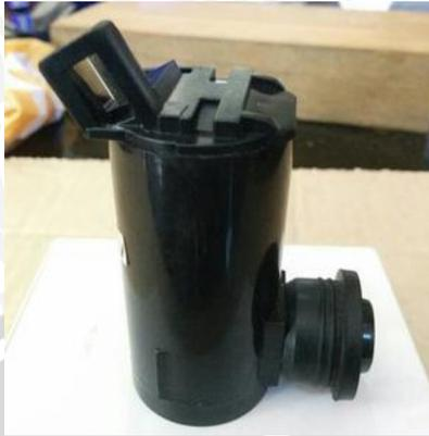
Gambar 2. 5 Pompa DC 12 V
