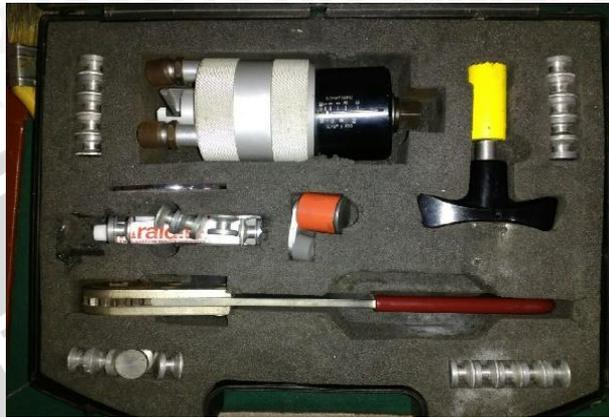
Gambar 3.2 Set alat *pull-off* ( *Elcometer 106* )
