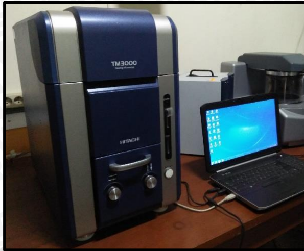
Gambar 2.13 Scanning Electron Microscope and Display SEM. Sumber: Laboratorium Sentral Teknik Mesin UB.
